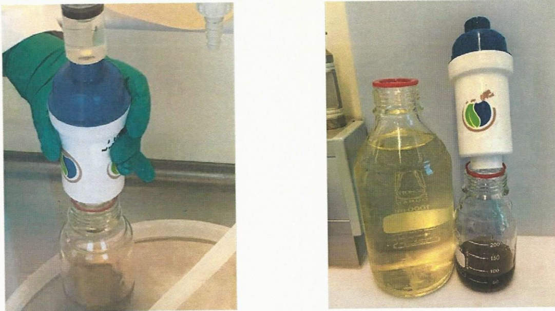
Fig. 3: Backflushing (image on left) and sample of effluent water (image on right)
